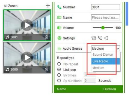
• Sound Device: two source, one is live microphone in, and the other one is the server could detect the signal from outside radio or music player like spotify and then auto
